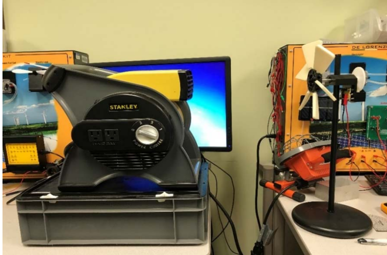
Figure 4: Experimental setup with a mini-wind mill mounted with six 3-D printed blades
