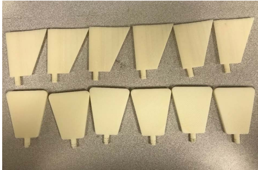
Figure 3: The actual 3-D printed curved and flat blades
