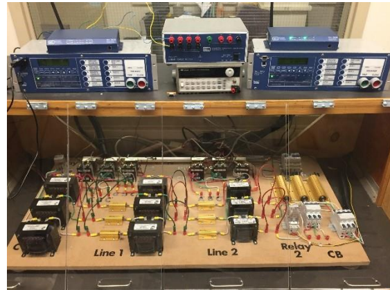
Figure. 2 Platform for digital relay experiments
