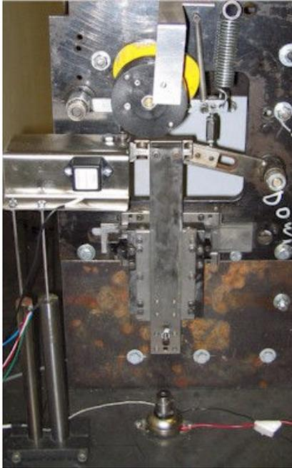
Figure 3 Cams with Sensors
