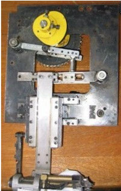
Figure 1 Cam Tooling from Gillette
