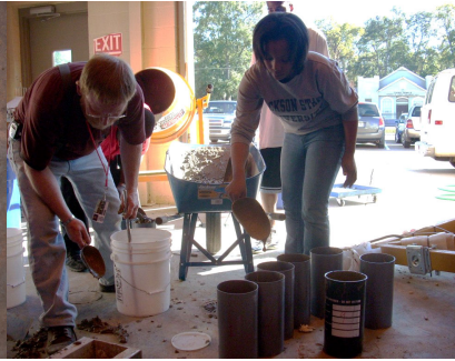
Fig.6 Students cast concrete specimen and embed iButton
