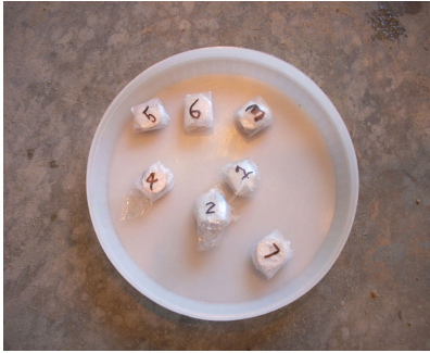
Fig.5 iButton sensors ready for embedding in concrete
