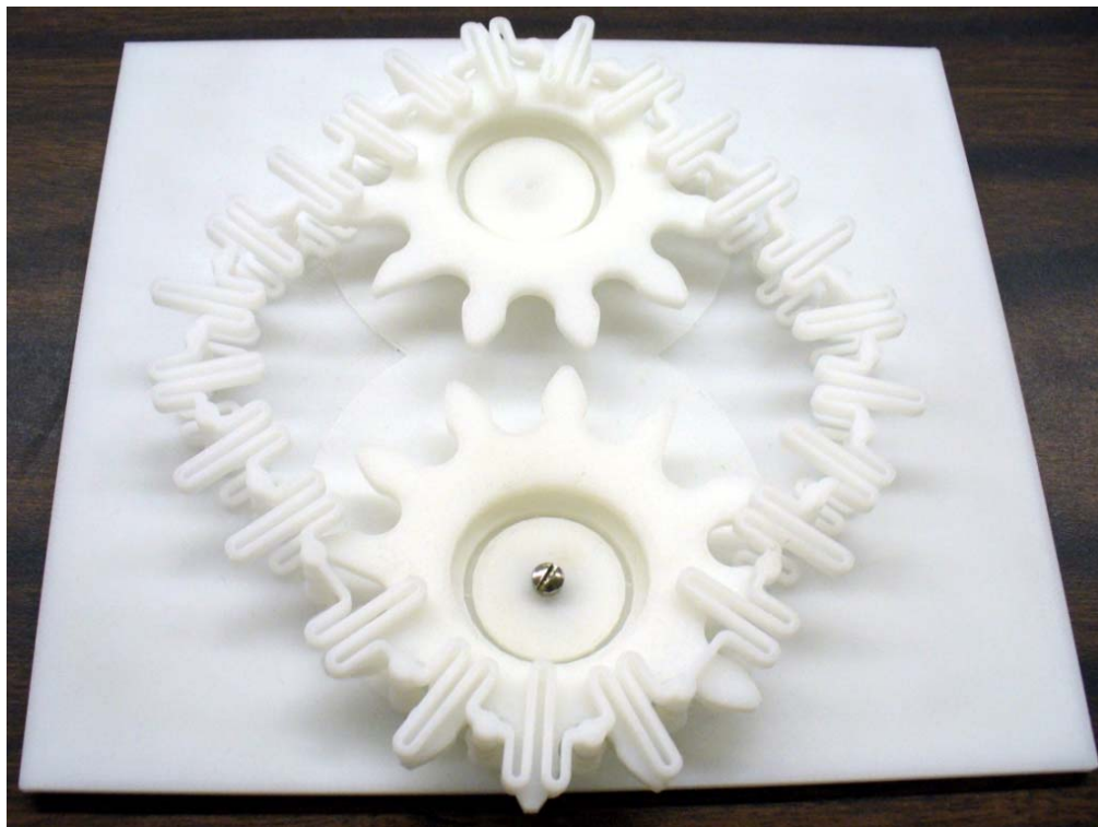
Figure 5. Rapid prototype of the Polysilicon belt design similar to the one shown in the previous figure.
