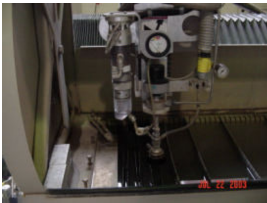
Figure 2. Cutting Head in WJC Equip.
