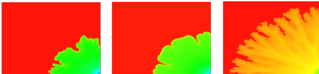
Fig. 8-Schematic showing simulated viscous fingering in water, oil, and mixed wet in a heterogeneous rock system.
