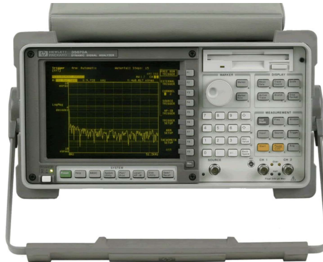
Figure 3. Dynamic Signal Analyzer (HP/Agilent 35670A) used in Linear Circuits labs.
