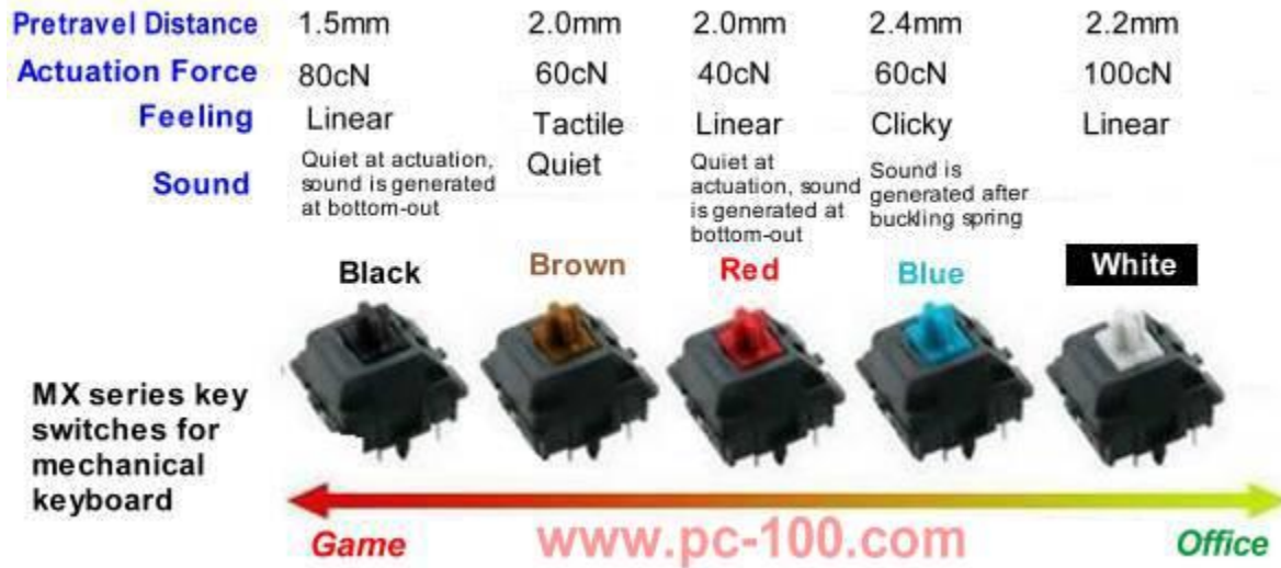
Figure: Commercially available mechanical switches with different required activation forces and tactile and auditory feedback
