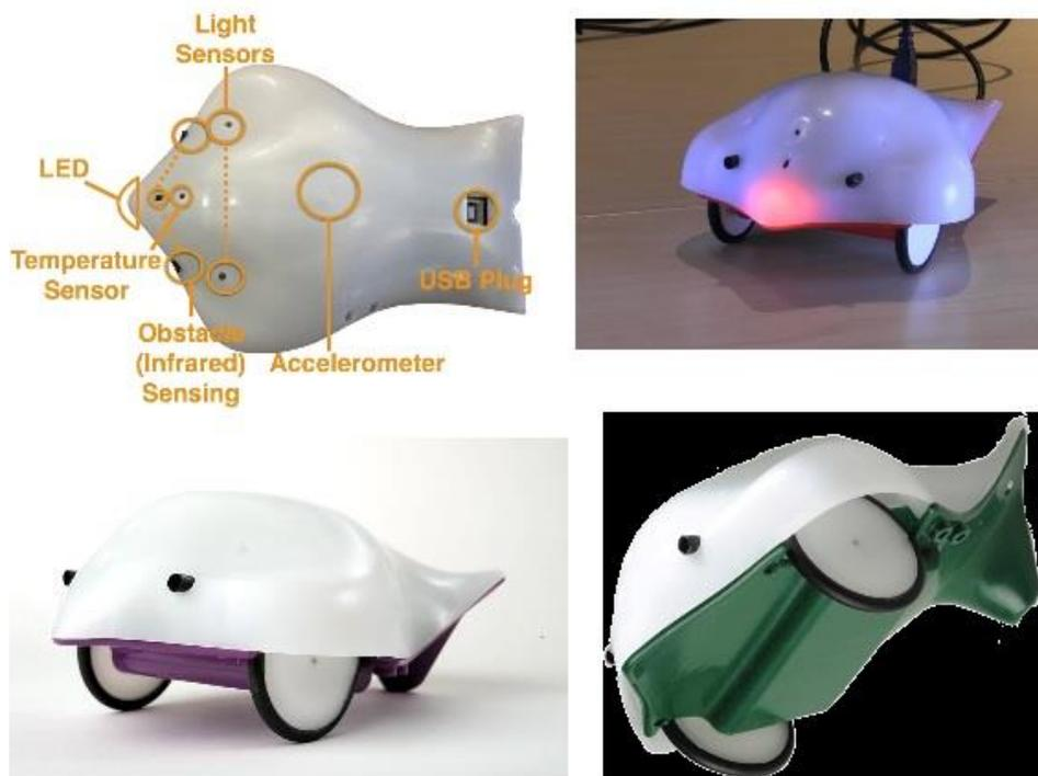
Figure 1: Finch Robot (courtesy of BirdBrain Technologies)
