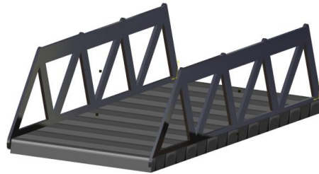
Figure 1: CATIA Design of a Warren Truss Bridge
