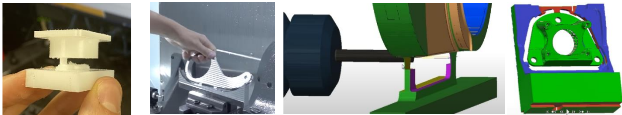
Figure 6. Examples of some different methods of CNC work holding: thick tabbing (a), thin tabbing (b), offset tabbing (c), and window machining (d) [8].
