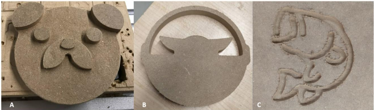
Figure 2: Example CAM router projects include (A) a dog face, (B) a baby Yoda, and (C) a bass. The bass project (C) is still embedded in the MDF board because the students did not define the profile cut around the boundaries of the model.
