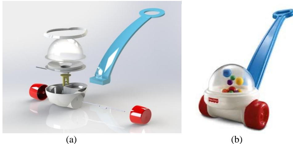
Figure 1. a) Solid Model constructed by student showing the exploded view of child's corn popper and b) picture of actual product.
