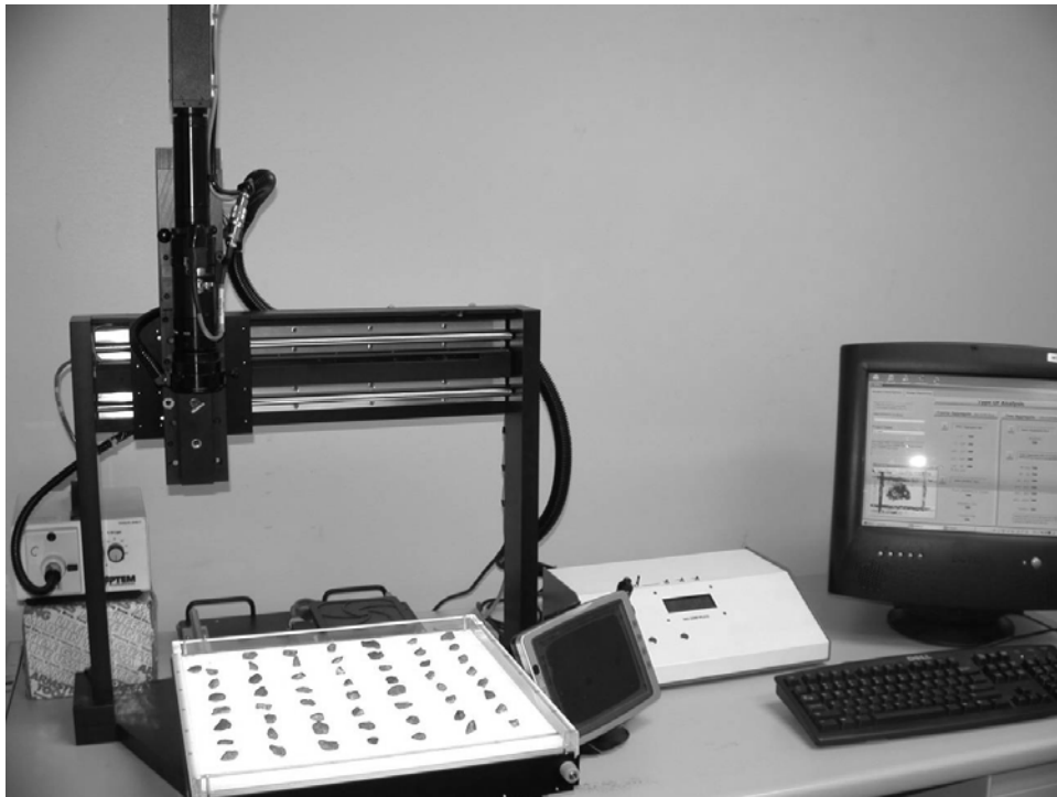
Figure 2. Existing Aggregate Imaging System (photo courtesy of Pine Instrument).
