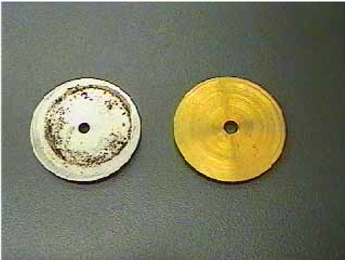
Figure 2. Two orifice plates employed by students to provide a load to the air compressor system (orifice plate on right is orifice plate design 2).
