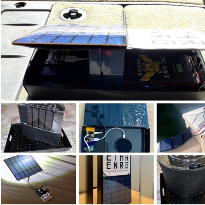
Figure 7: ETHR-ENRG Smart Solar Novice, Intermediate, and Advanced Project Kits Assembled And Working Properly
