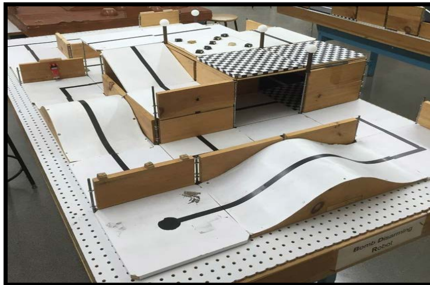
Figure 2: Autonomous Robot Terrain with Obstacles that Represent Real World Scenarios
