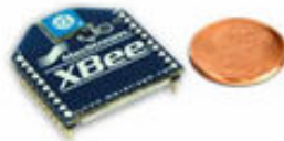
Figure 2. Digi/MaxStream XBee 802.15.4 radio modem with a chip antenna
