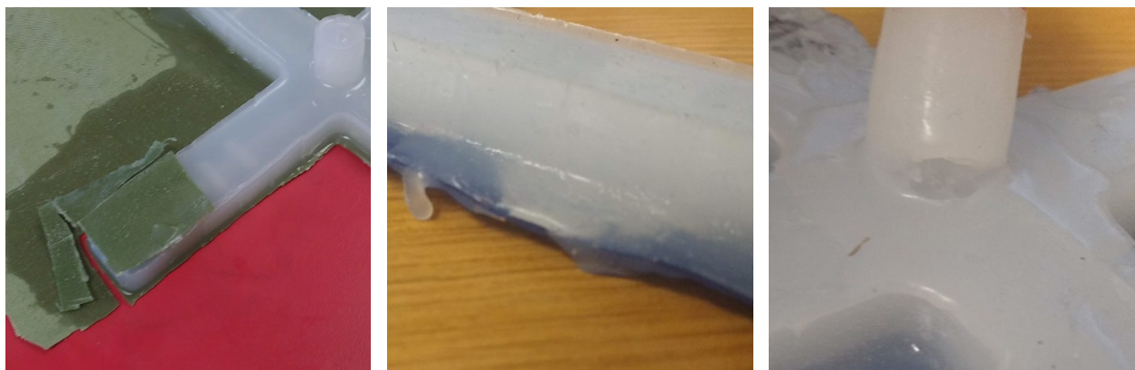
Figure 10. Fabrication flaws experienced by Sydney and Jordyn: 1) leaked mold leading to holes in the top surface (patched unsuccessfully); 2) poor adhesion between layers leading to leak on side; and 3) clogged air chambers leading to a rupture near air inlet.
