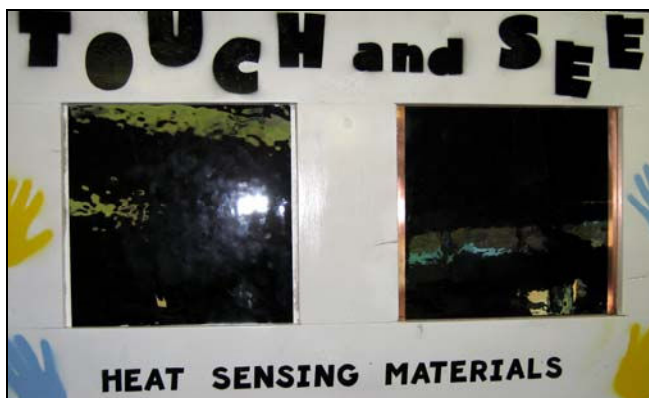
Figure 7. The two liquid crystal panels show different backings: Styrofoam (left) and copper (right) produce different effects due to different thermal conductivities and heat transfer rates.
