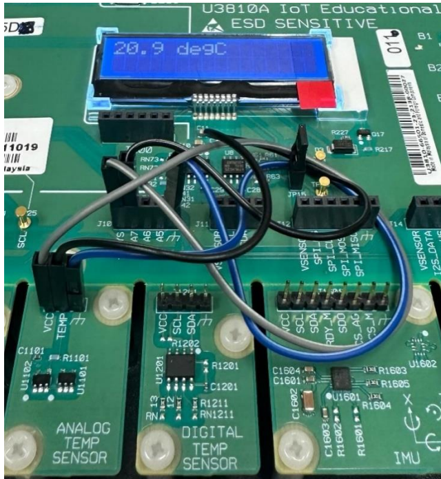
Figure 6. Temperature values output to LCD display.
