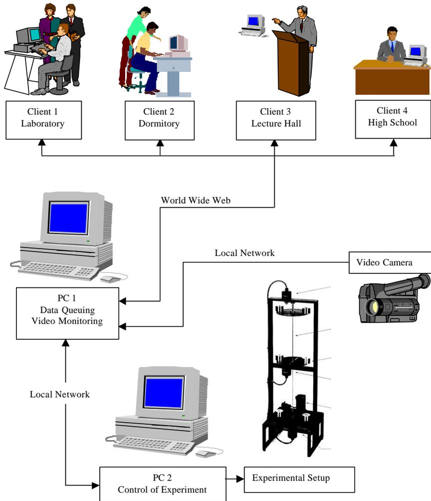
Figure 1: Setup of undergraduate laboratory
