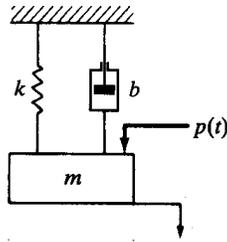
Figure 4: Schematic representation of a one-degree-of-freedom forced vibration system
