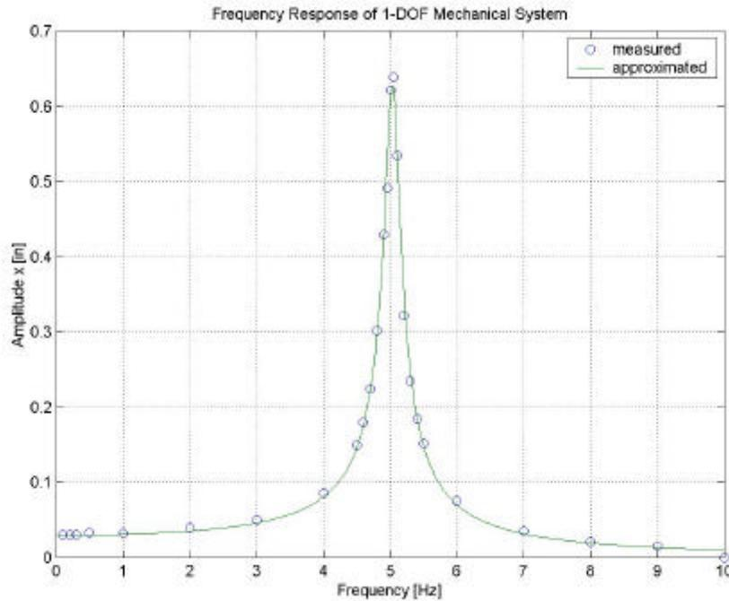
Figure 6: Frequency response for one-degree-of-freedom mechanical vibration system
