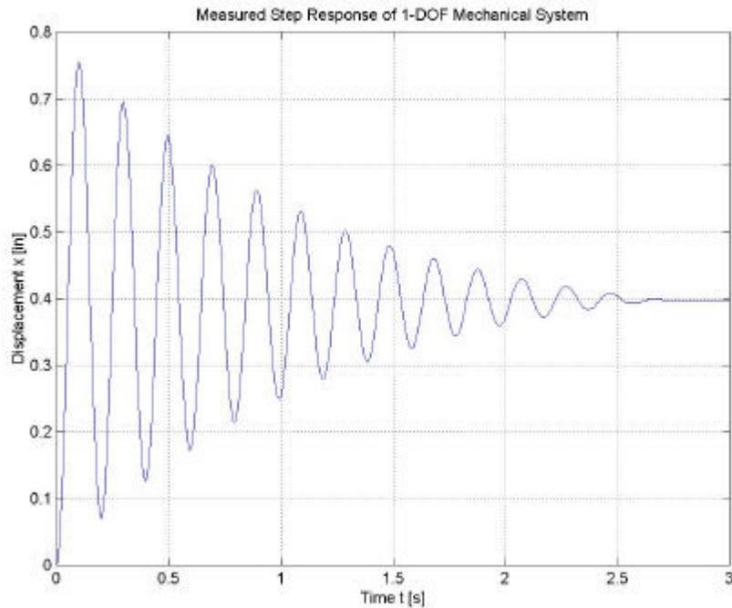
Figure 5: Measured step response for one-degree-of-freedom mechanical vibration system
