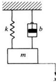
Figure 2: Schematic representation of a one-degree-of-freedom free vibration system
