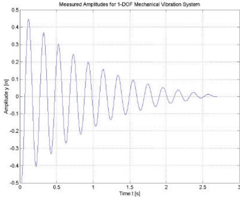
Figure 3: Measured amplitudes for one-degree-of-freedom mechanical vibration system
