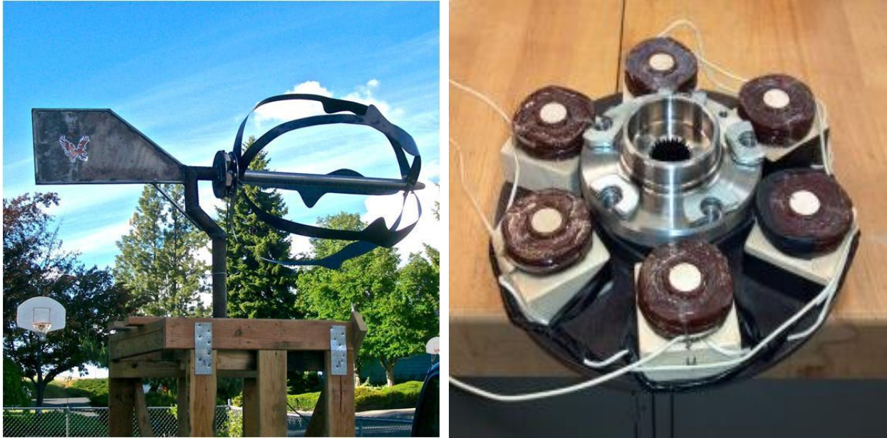
Figure 5 The energy ball style windmill and coils mounted in the generator.
