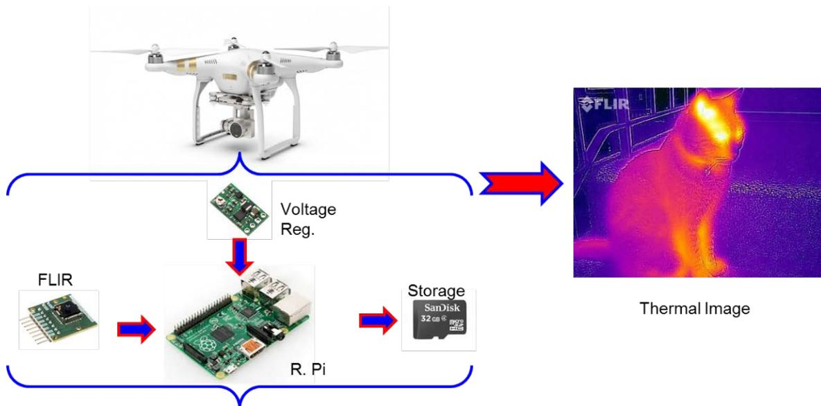
Figure 1. Low-Cost Thermal Sensor Payload System Diagram
