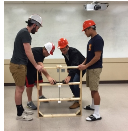
Figure 2. Photo of students loading the demonstration. Two students are used to help support the frame and two students simultaneously load weights - alternating between the top and bottom spans.
