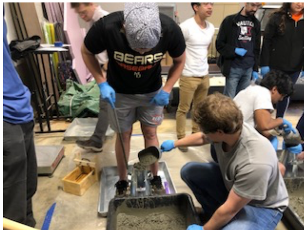
Figure 2: Students mix concrete, grout and mortar
