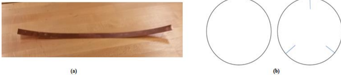
Figure 2. (a) copper fin and (b) unfinned and finned pipe sectional sketches
