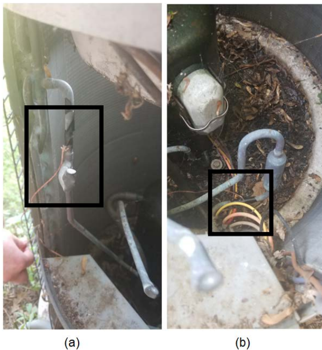
Figure 1. Thermocouples wrapped on the refrigerant pipes across the condenser
