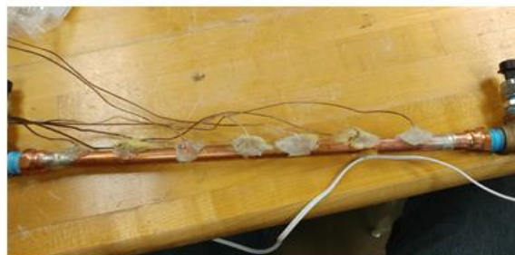
Figure 4. Thermocouples embedded into the center of the testing section
