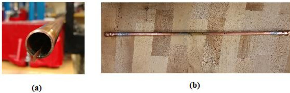
Figure 2. (a) inner fin soldered into the inner surface of the testing pipe and (b) testing section copper tube with holes made for thermocouple
