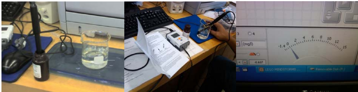
Figure 4: Calibration steps of Dissolved Oxygen Sensor at UMES Lab
