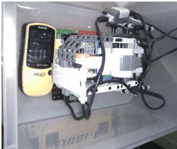
Figure 2 a. Mechanism to toggle GPS switch
