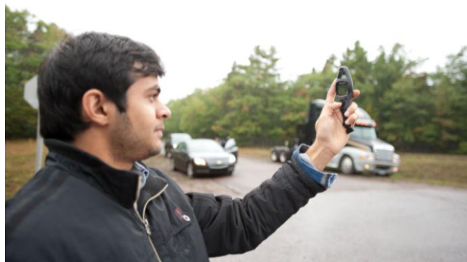
Figure 4: In-Situ measurement of environmental conditions. Measurements obtained included wind speed, air temperature, humidity, and barometric pressure.
