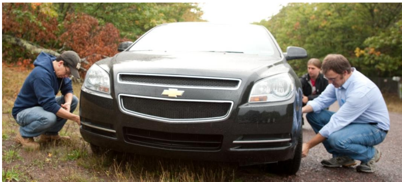
Figure 2: Tire pressure adjustments being made at the mustering location between coastdown runs.
