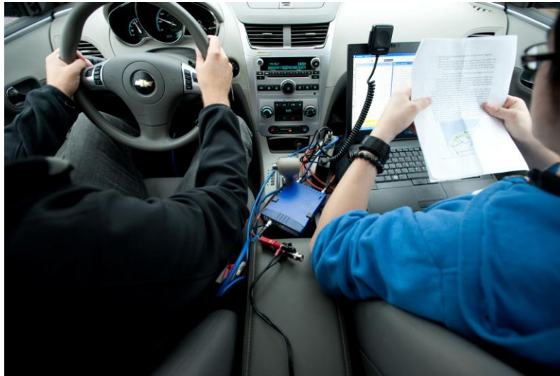
Figure 1: Students conducting a coastdown test.
