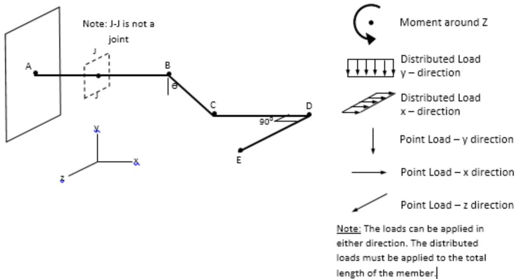
Place 4 of the 6 loading situations on the above structure to result conceptually in the maximum value at plane J-J for each of the following stresses. Loads can only be added to joints and can be either in the positive or negative direction.
