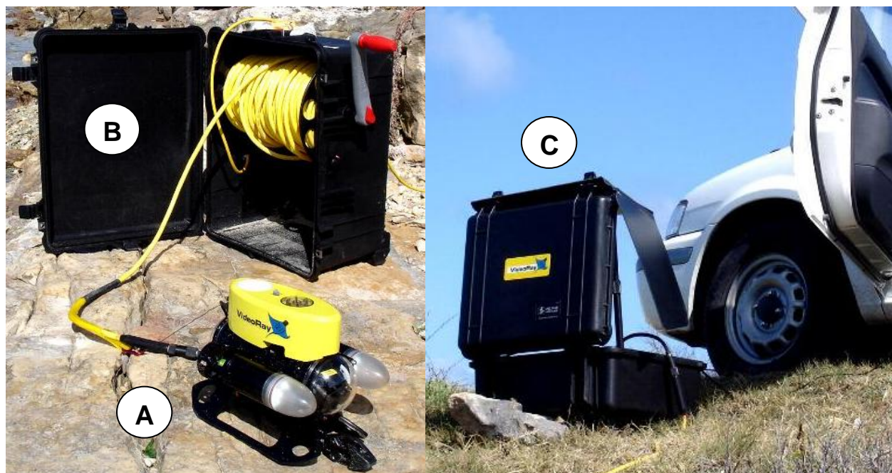
Photograph 1: Typical VideoRay ROV Setup for Shore Accessible Site; (A) Submersible, (B) Tether, and (C) Control panel. Inverter not shown.
