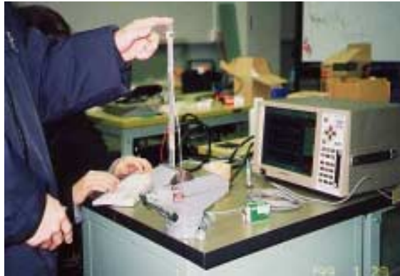
Figure 18 Measurement of Strain and Acceleration on Aluminum Plate
