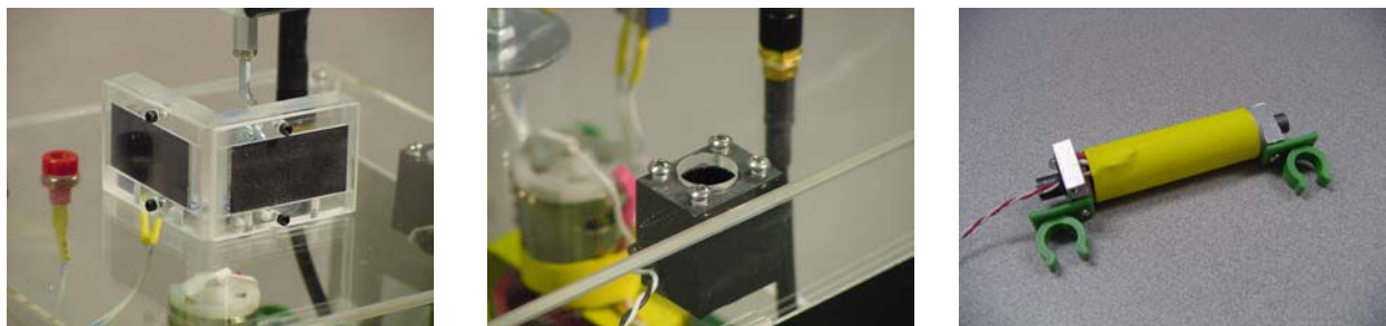
Figure 12. EyasSAT attitude sensor, sun sensor, and torque rods
