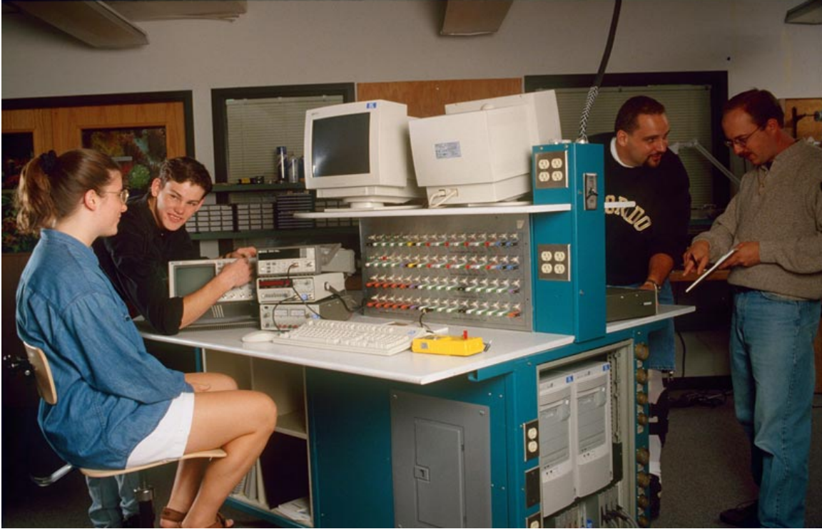
Fig. 1. ITLL LabStations provide powerful computer and data acquisition capabilities for two teams of students to conduct hands-on experiments in the open lab plazas.
