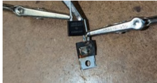
Figure 2: Transient test result of a power MOSFET.
