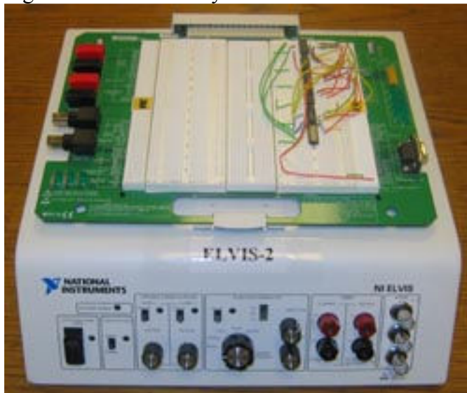
Figure 2 – NI-ELVIS system with a breadboard circuit.
