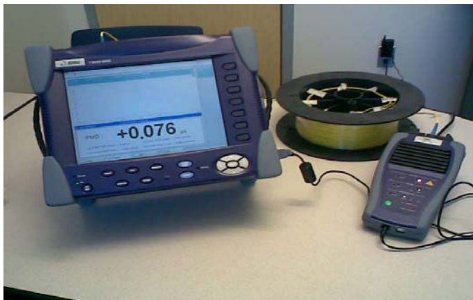
Figure 5 Experimental setup for PMD measurements
