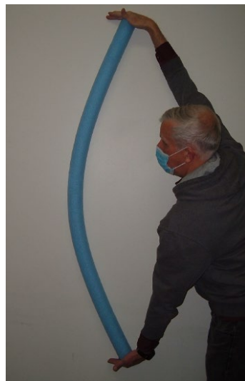
(a) Pinned-Pinned Ends
