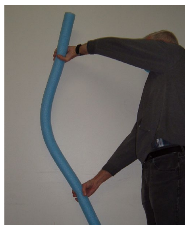
(b) Long column “buckling” behavior
