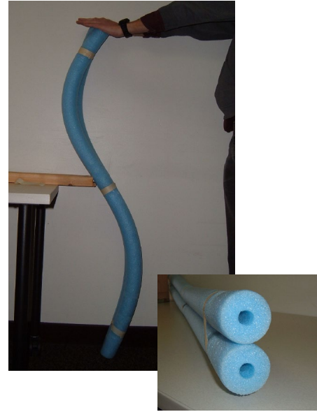
Figure 9 – Effect of Bracing on Buckling Length
