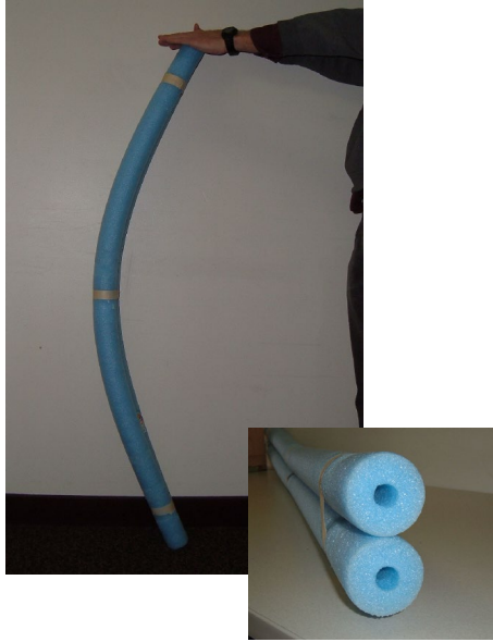
Figure 8 – Effect of Moment of Inertia on Buckling Direction
