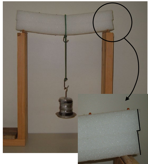
(b) After Shear Failure
