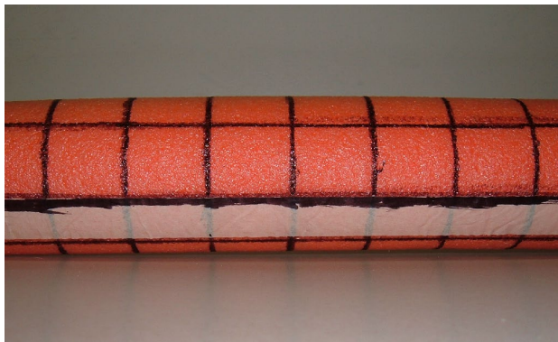
Figure 4 – Deformation of Shaft due to Torque
