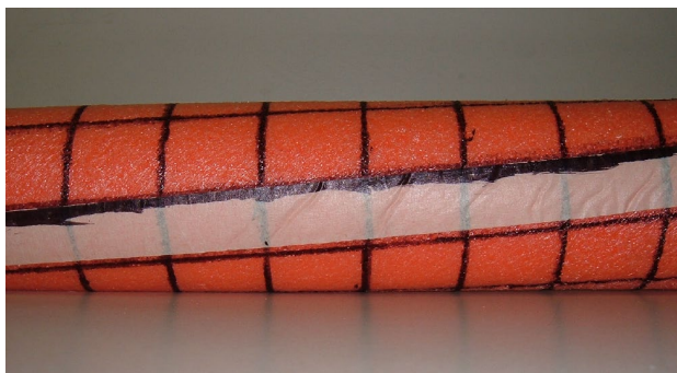
Figure 5 – Torsion Demonstration with Pool Noodle
