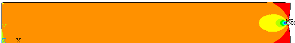
Fig. 7 A Typical FEA Post-Processing Graph for a plate under compression to illustrate Saint Venant's Principle.
