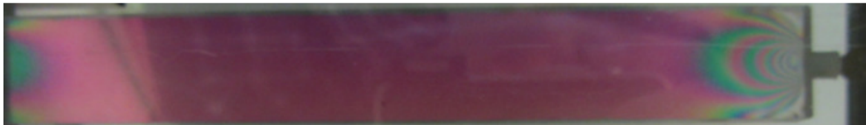
Fig. 3 A color map for an axially loaded bar in the Stress-Opticon Kit.
