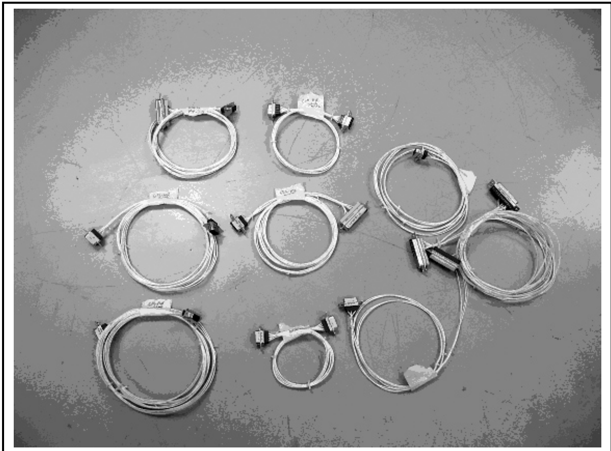
Figure 7. Wire Harness Before Installation
