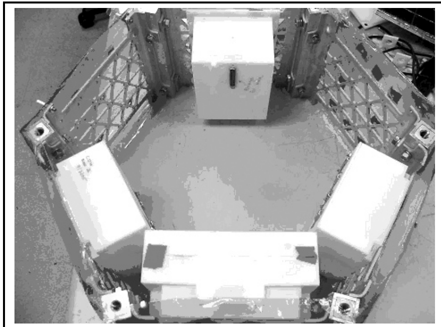
Figure 12. FASTAC Satellite with Four Prototype EMI Boxes Integrated
