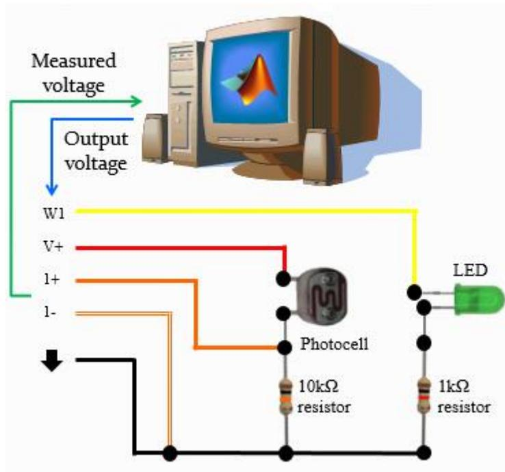
Figure 1: Schematic of a DAQ Experiment in Models I
