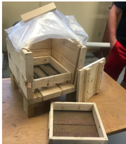
Figure 4. Completed Phase 2 solar-powered food dehydrator design #1; food trays are stackable.
