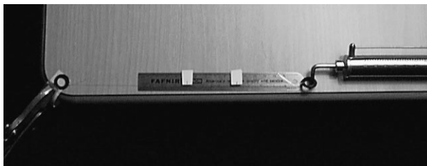
Photo 1 - Testing with spring gage, washers on both ends of sample.
