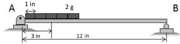
Figure 5: Uniformly distributed load that provides equivalent reactions to Figure 2.
