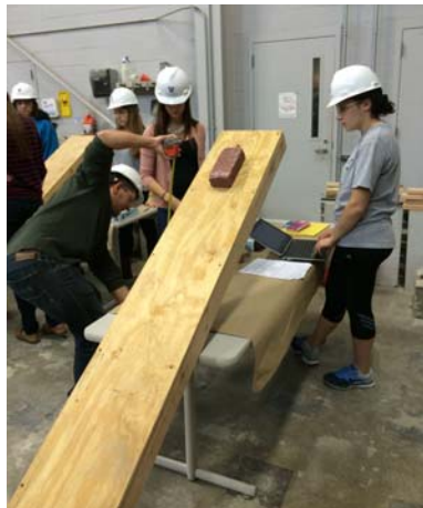
Figure 13 – Student group conducting coefficient of static friction experiment
