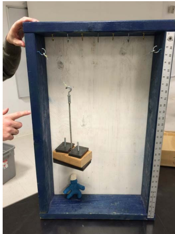
Figure 2 – Loading rig for fishing line exercise
