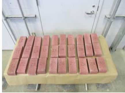
Figure 11 – Set of numbered bricks for friction laboratory exercise
