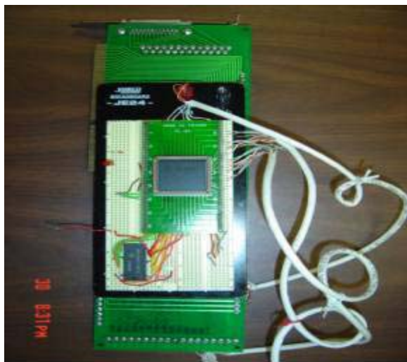
Figure 6. “Programmed” version of the controller circuit using the XC95108 CPLD
