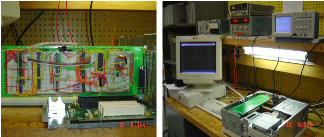
Figure 4. Prototype breadboard (left) of the ADC/DAC controller circuit inserted in the EISA bus slot of the PC (right).
