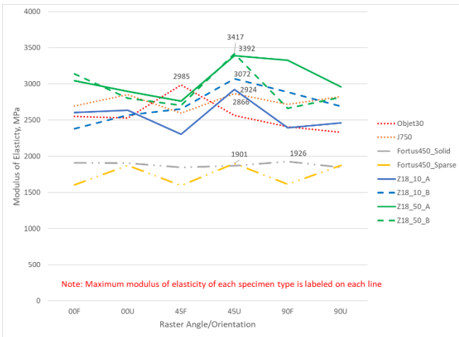
Figure 14. Modulus of Elasticity of All Specimens
