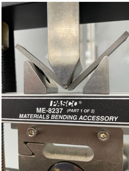
Figure 9. Specimen Failure During Testing
