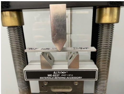
Figure 8. Specimen Mounted on Test Stand
