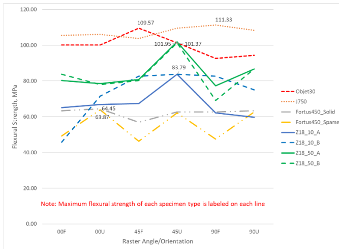
Figure 21. Flexural Strength of All Specimens
